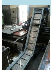
The channels can be single or double for monoor bi-material. In this case, a vane channel for brass and one with shutters for steel have been created.
