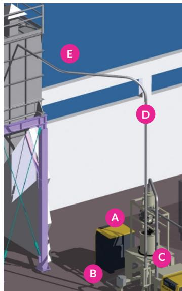
FAMA **pneumatic delivery systems** feature the maximum versatility and extensibility and are suitable for any type of swarf, as long as they are short and dry.
