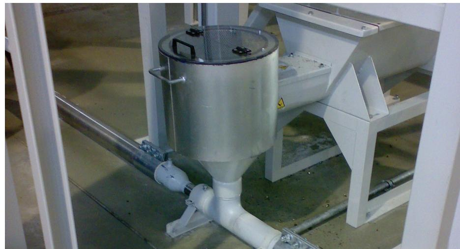
In the case of a single silo, the inlet is direct. In the case of double or triple silos, the wood chip inflow is managed by a cyclone separator, which feeds a paddle conveyor used to redistribute the chips into the various silos
