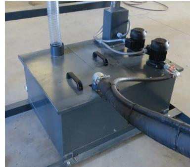
**Swarf and oil collection and treatment tank:** the coolant and oil/emulsion collected by the machines are sent to this tank. The dredger extracts the swarf deposited on the bottom. Pump1 sends oil to the channels for swarf flushing and transportation, pump2 sends oil in low pressure to the machine, pump3 sends the oil to the filter, pump4 sends oil in high pressure to the machine, pump5 is used for the filter self-cleaning system.
