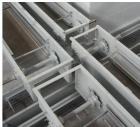
Changes of direction can take place by gravity (1), or by direct intersection for the oil and with duck beak for the solid part (2).
