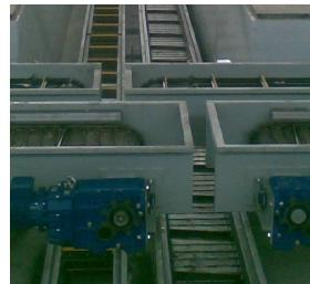
The channels can be single or double for mono or bi material. In this case a paddle channel was created for brass and a roller shutter channel for steel.
