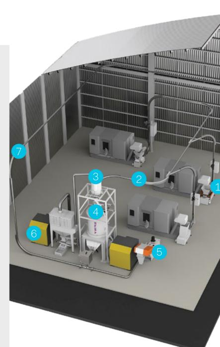
The metal chips exiting the machine tool's evacuator are collected in the GSM. When the desired level is reached, a sensor initiates the vacuum process. Within seconds, all material is transferred to the cyclone separator and falls into the centrifuge.
