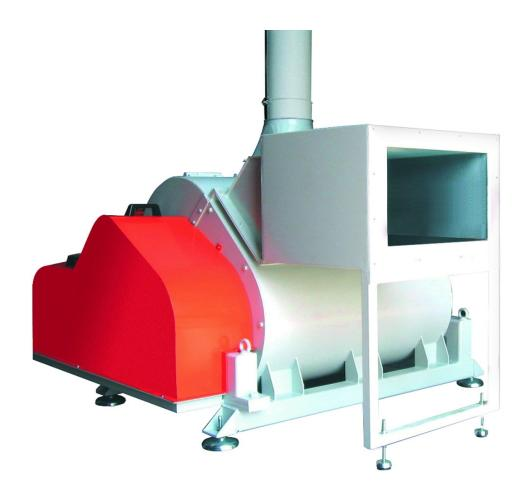
The "LUPO" model shredder is a sturdy machine consisting of a shredding chamber and two shafts rotating at different speeds with shredding rotors with spokes complete with interchangeable blades.
