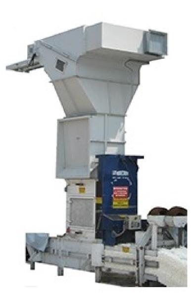
The "PSC" grille separator is a static element studied and designed for the separation of paper, cardboard and aluminium waste from the air, in pneumatic conveyor systems.
