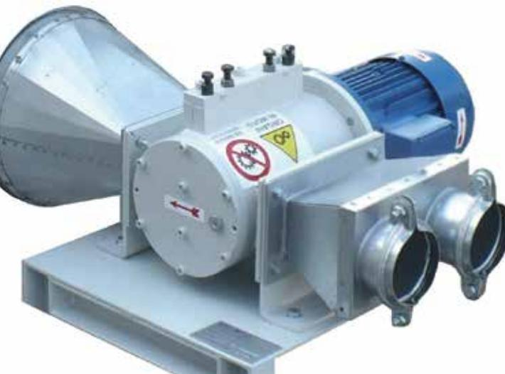
*This machine has been developed and designed to be installed on extraction systems serving machines which produce problematic trimmings such as plastic packing film, polythene and aluminium foil. Entirely machined with precision mechanics, the cutter shreds the trimmings directly on the machine, so they can be transported by a pneumatic conveyor.*
